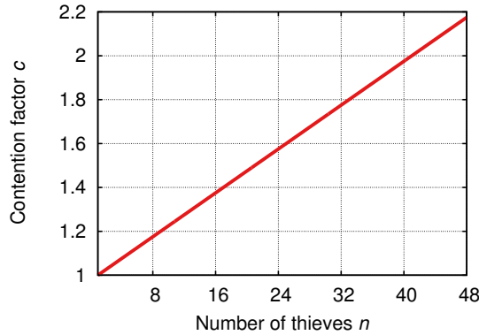
Figure 3.7: When steal requests cause contention among thieves, the overhead of last-victim selection may exceed that of random victim selection if the time required to send a steal request increases by more than a factor of c . The graph shows how c increases with the number of concurrent thieves, assuming that steal requests are 5% more expensive to send than tasks. (Steal requests use MPSC channels, whereas tasks use faster SPSC channels.)
